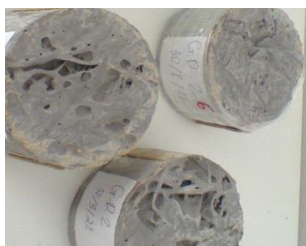
Fig. 3 – Sample geopolymer material for exhaust ventilation
